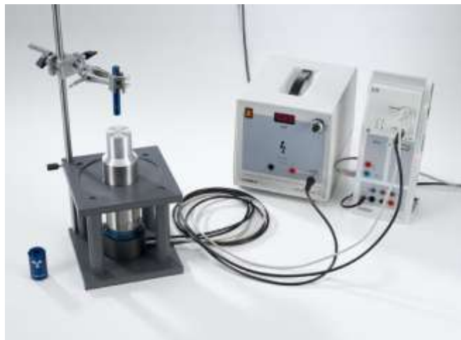
Figure 2. Experimental Setup for Gamma Radiation Detection Using a Scintillation Detector
